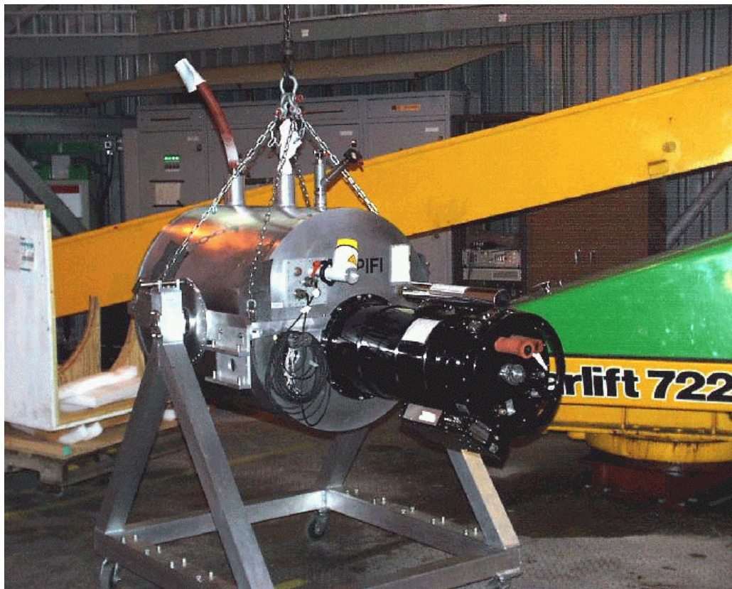
Frontispiece: Top: the new central bearing housing safely installed under the main support axis of the antenna. Instrument; Bottom: SPIFI assembled on the carousel floor awaits hoisting to the Nasmyth platform.
